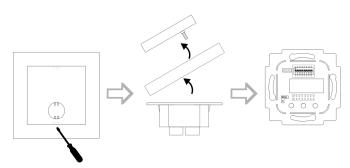
The device is designed for mounting on a flush box. The bus cable is connected to the device by a terminal screw. For pre-wiring, the terminal screw can be drawn from the device.
