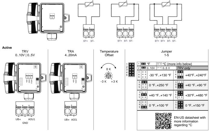
fig. (Measuring range and offset adjustment, default settings: +40 °C..+240 °F | 0 K)
