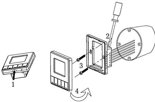
For Installing or repairing, please make sure the power is disconnected. Insert the screw driver in the plastic teeth of thermostat. Clockwise rotation of the screwdriver will separate front cover from base plate. Please follow the wiring diagram to connect the wires. Fix the thermostat base plate to the wall through the four screw holes with distance between axes of 60 mm. Fasten base plate and front cover. Do not press the panel in order to protect LCD.
