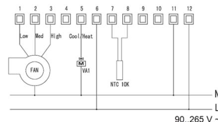
Wiring diagram for 4-pipe fan coil
