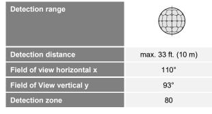
A installation height of 16.4 ft. (5 m) results in a detection area of approx. 52.1x40.3 ft. divided into 80 measuring zones.
