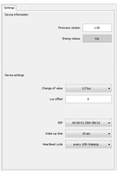
The device information shows the installed <u>Firmware version</u> and the current <u>Energy status</u> of the device is full charged or a battery is inserted. The Energy status must be **OK** to configure the device.
