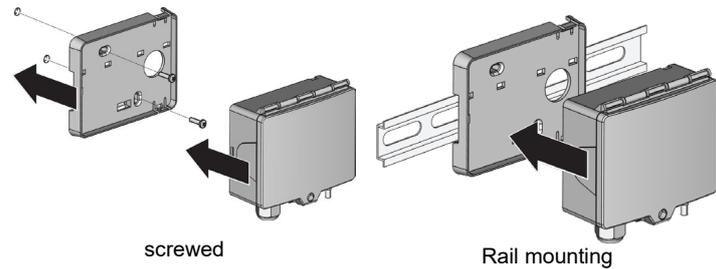
**2.** Prepare the duct for mounting and mount the duct connection piece. **Attention! Observe dimensions!**
