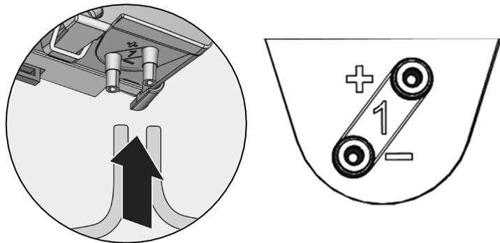
**4.** Connect pressure tubes to the duct connection pieces
