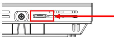
Position of the micro USB port, see bottom of the device, for configuration with Bluetooth dongle or Micro-USB programming interface
