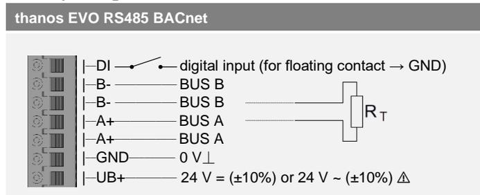
With alternating voltage, the correct polarity must be ensured! Please note the technical data.
