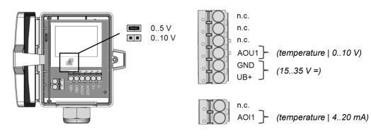
AKF10+ (LCD) TRV MultiRange Relay
