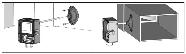
Optional mounting with mounting base (Item No. 631228), please note the installation depth of the sensorpocket. (permissible ambient temperature -35..+70 °C)
