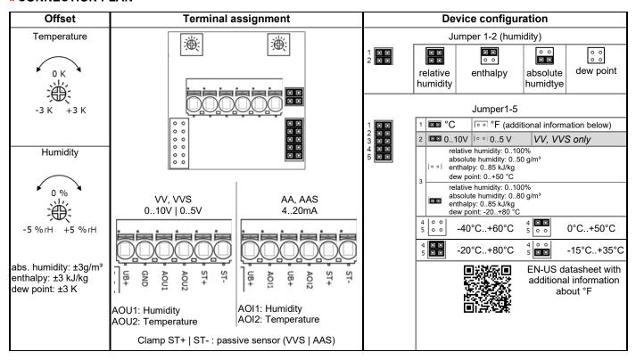
The adjustment of the measuring range is made by changing the jumpers in a de-energized state. The output value of the new measuring range is available after 2 seconds. fig. (Measuring range and offset adjustment, default settings: -20 °C..+80 °C | 0 K)
