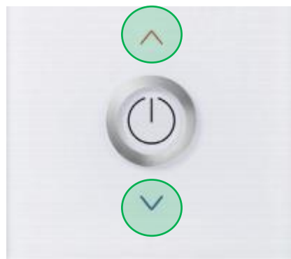
Picture 10 Key combination HC type for invoking modbus settings menu
