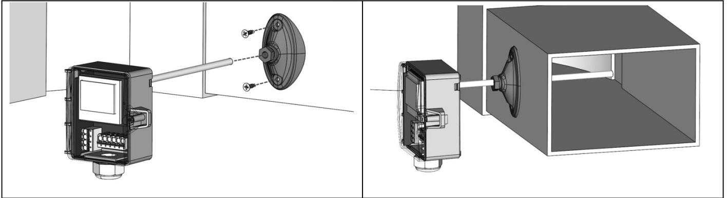
**Optional mounting with mounting base (Item No. 631228), please note the installation depth of the sensorpocket.**
